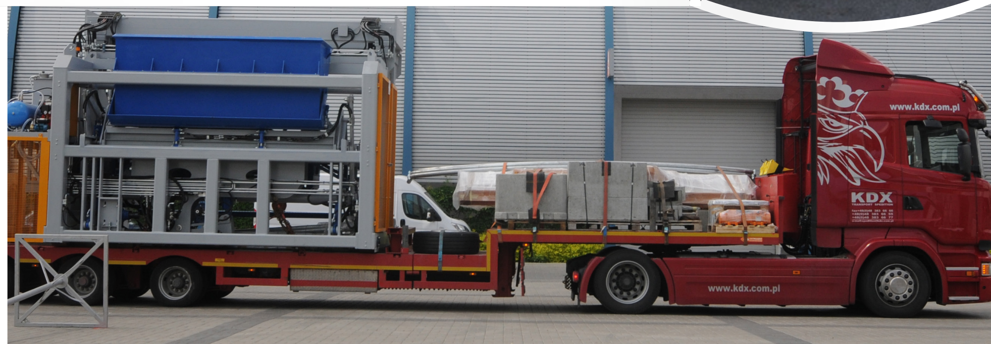
The VibroCast™ machines can be carry on truck as special transport without escort (max width mt. 3,0) or inside the container disassembled for long marithime transportation.
